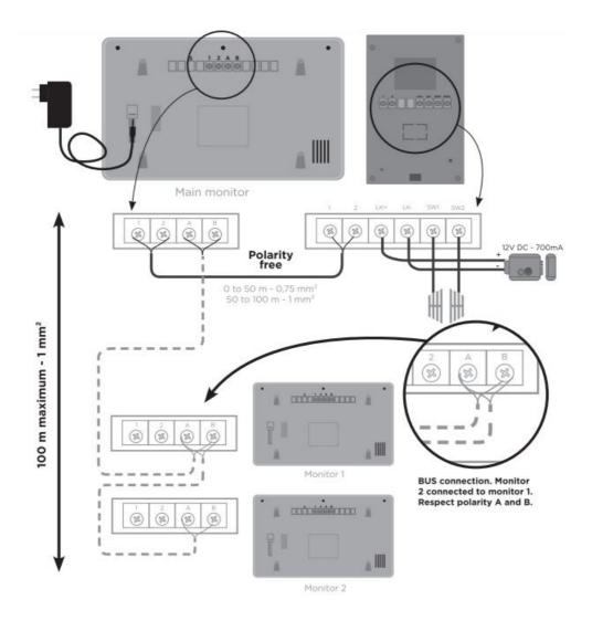
You can directly connect the monitor to your electrical panel via a 15V DC 0,8A (minimum) «rail DIN» transformer. Electrical knowledges are necessary, in this case. Please contact a professional.
