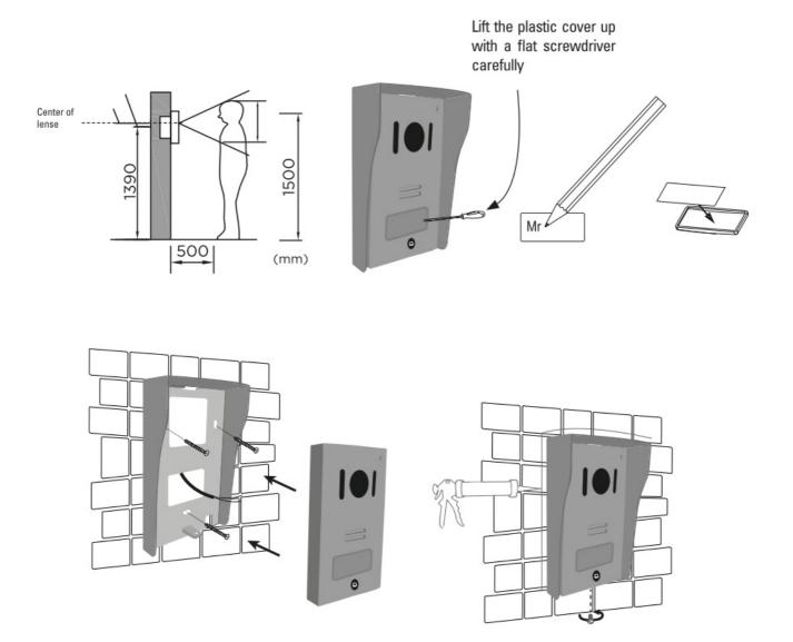
After installing and test, place a transparent acid free silicone seal at the top and on the sides of the door station (not at the bottom) to avoid any risk of infiltration.
