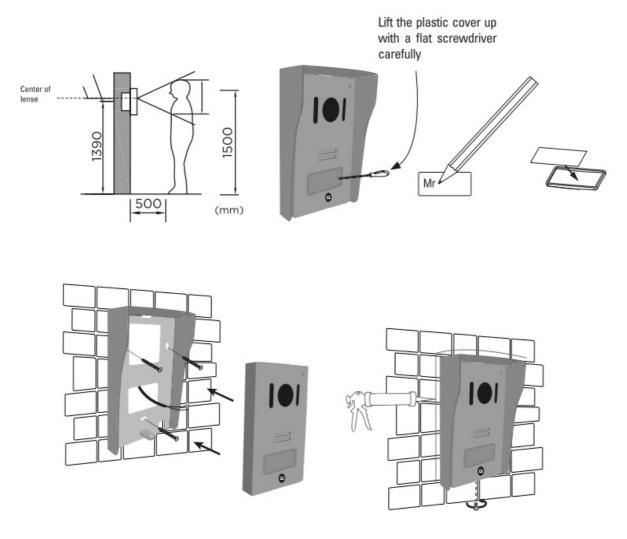
After installing and test, place a transparent acid free silicone seal at the top and on the sides of the door station (not at the bottom) to avoid any risk of infiltration.
