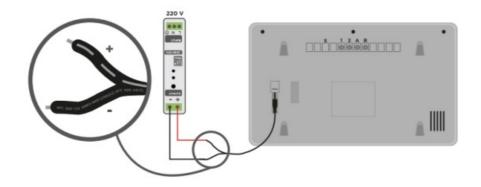
**B2- Installing** Indoor monitor
