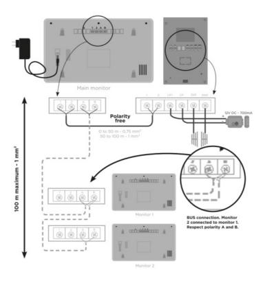
You can directly connect the monitor to your electrical panel via a 15V DC 0,8A (minimum) «rail DIN» transformer. Electrical knowledges are necessary, in this case. Please contact a professional.
