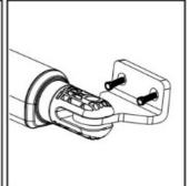
Make sure arms are fixed in horizontal position especially in those positions: 1) Gate in « CLOSE » position 2) Gate in « OPEN » position 3) Gate at « 45° angle » position Prior to weld the bracket on the gate leaf (if necessary), cover the gate opener to prevent damages from sparks.
