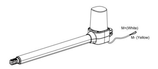
Avoid tension in the cable during open and close phase. For gates opened outward: M1 Motor: Connect the motor wire (Yellow -) to the terminals Mo1 + and (White +) to the terminals Mo1 - and (White +) to the terminals Mo2 - and (White +) to the t
