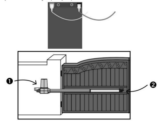
1. Fix the first bracket to the pillar. Position the automation in the bracket, then place the screw and nut.
