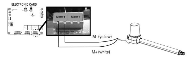
M2 MOTOR CONNECTION (second opening motor)
