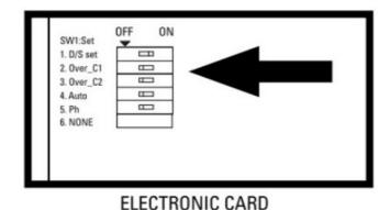
Switch settings: «on right position, «offy left position. DIP SWITCH 1 D/S set: ON = double gate operation OFF = single gate operation (connection on 11 and 12)
