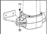
2. Assemble the second bracket with the other side of the automation and screw the bracket to the closed gate.
