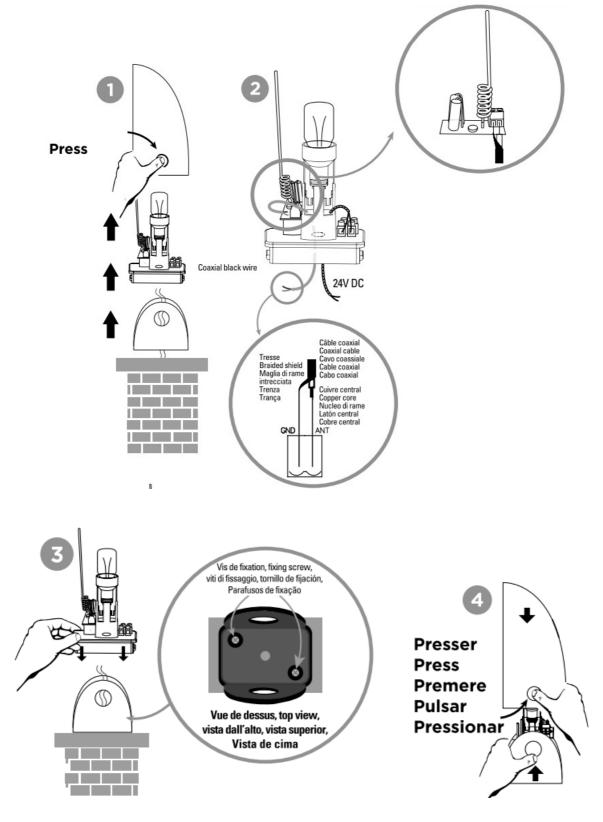
If you want to improve the operating range of your remote, you can connect the blinker antenna with a RG58 coaxial cable (not supplied). In this case you must disconnect the original antenna and then connect the coaxial copper core to the terminal ANT and the coaxial braided shield to the terminal GND on both antenna and electronic card.
