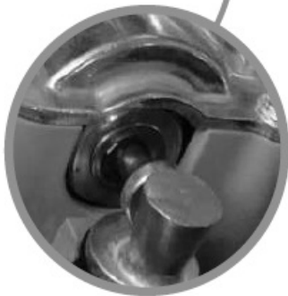
Position of locked motor : the pinle should be exited
