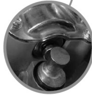
Position of unlocked motor : the pinle should be pressed
