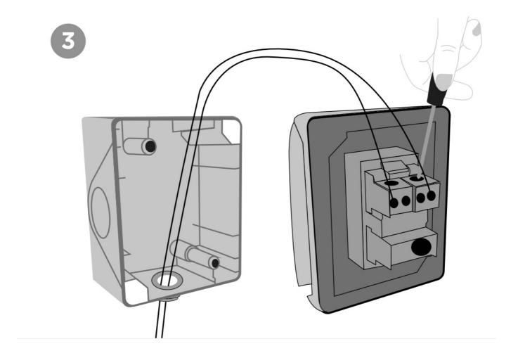
1/ Let's be sure it is disconnected from the mains. 2/ Connect the two wires for mains 230V on a surge protector plug with fuse or circuit breaker (installation compliant with standards in force: NFC 15 100 in France). 3/ The section of wires connected to 230 V must not be lower than 1,5 mm•.
