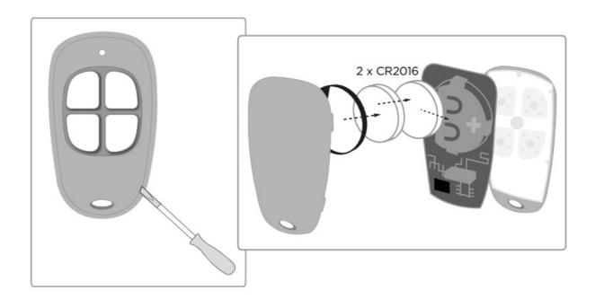
To change the batteries, use 2 x CR2016 batteries. Follow the diagram to open the remote and replace the batteries.
