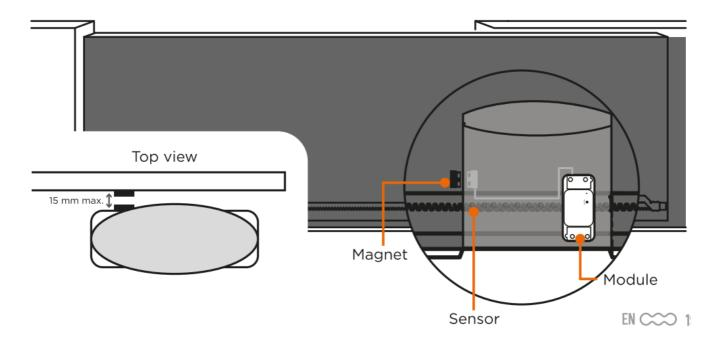
The module uses the magnet and sensor to indicate whether the gate/door is closed or not.
