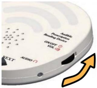
To shut off the unit, turn the thumbwheel counter-clockwise until you hear a click.
