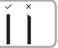
• We recommend only using the Reverse button when removing and changing filament. If only partially withdrawn, filament can swell in the pen and create jams. If this happens, fully withdraw the filament and cut the swollen part off.
