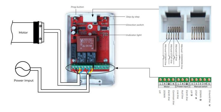
$\triangle$  The working mode for external manual switch is no power dry contact mode, the function of this two interface is the same.
