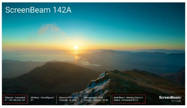
**Wifi Direct:** After the MultiBeam feature is enabled, a hidden AP is created on the Primary receiver, and the Remote receiver will connect to this hidden AP by wireless when MultiBeam Interface is set to **Wifi Direct**.
