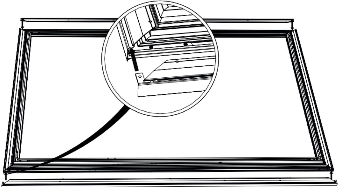
2. Push the trim corners flush and hold while tightening the set screws. Add, two per corner, of the 1/4-20 x 1/4" trim screws and verify corners are flush. Split Frame Only: Connect the horizontals at the middle by installing quantity 4 1/4-20 x 1/4" screws trough the trim into the splice bar.
