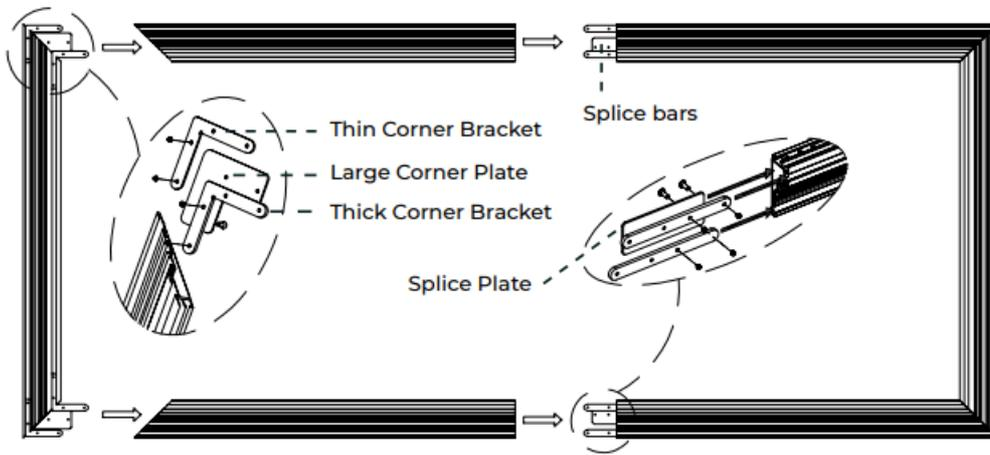
3. Align the frame corners to be flush and 90 degrees before loosely tightening one set screw on either side of the corner (on each corner of the frame) the frame must be square before fully tightening frame screws
