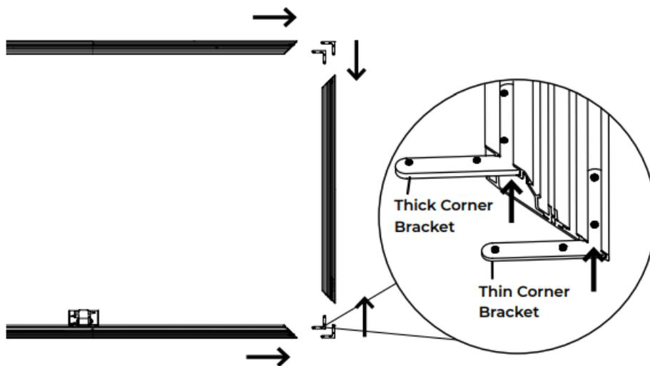
3. Align the frame corners to be flush and 90 degrees before loosely tightening one set screw on either side of the corner (on each corner of the frame) the frame must be square before fully tightening frame screws
