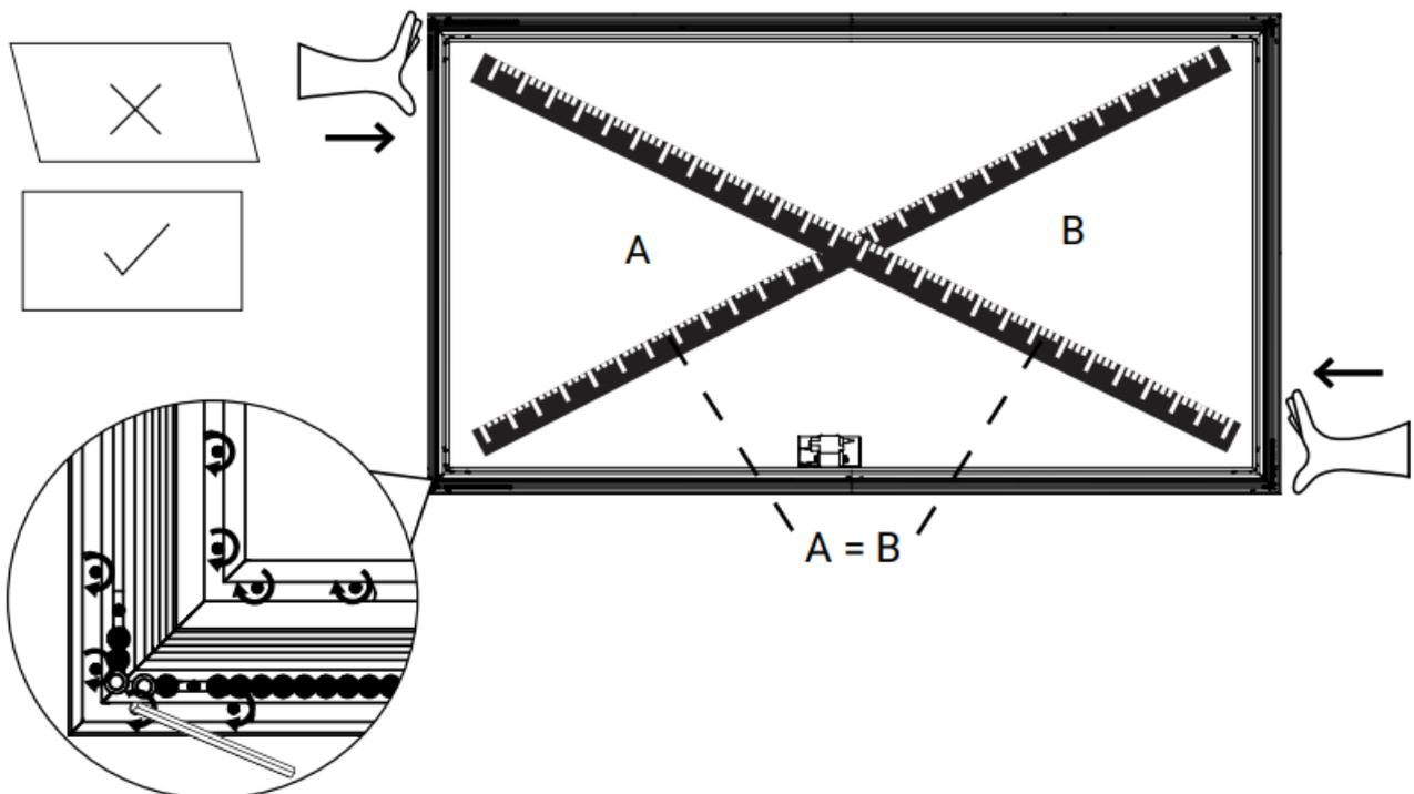
5. Install the vertical support bar by aligning the channel plates to be roughly centered on the frame, loosely screw the support bar to the channel plates and adjust to square by measuring top and bottom to the same vertical frame before tightening fully.
