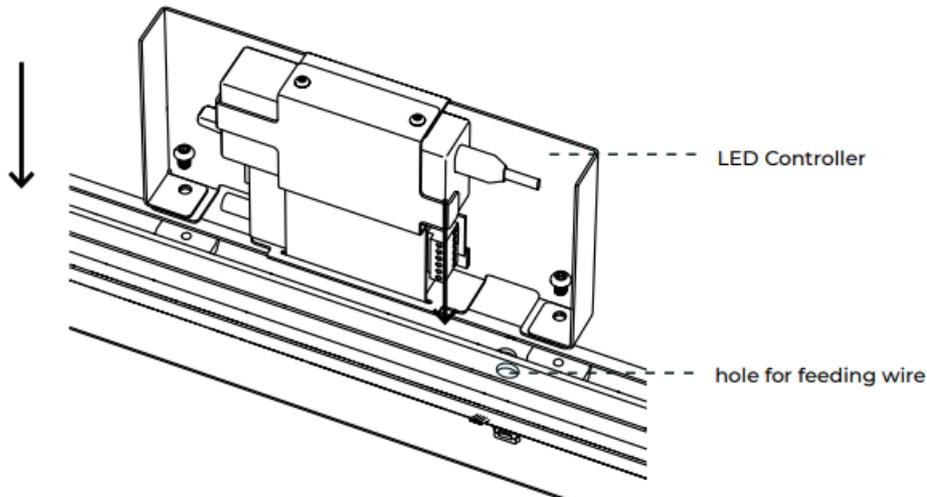
2. Feed the wires through the hole
