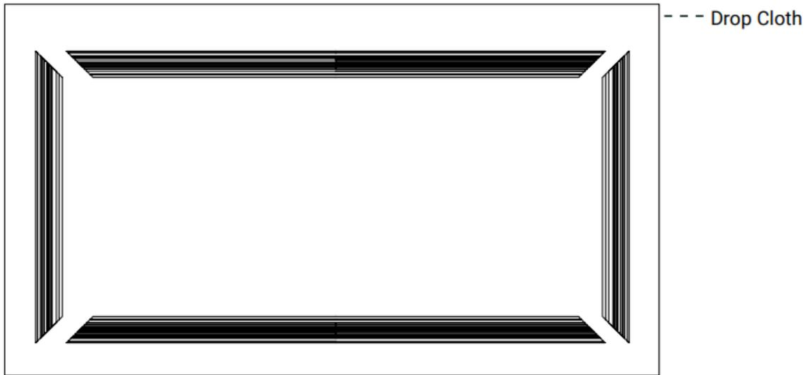
2. Insert the corner brackets as shown in the diagram, both thin and thick corner brackets have the same profile but as implied, one is thinner than the other. The thinner bracket is used in the channel closest to the outer frame edge.
