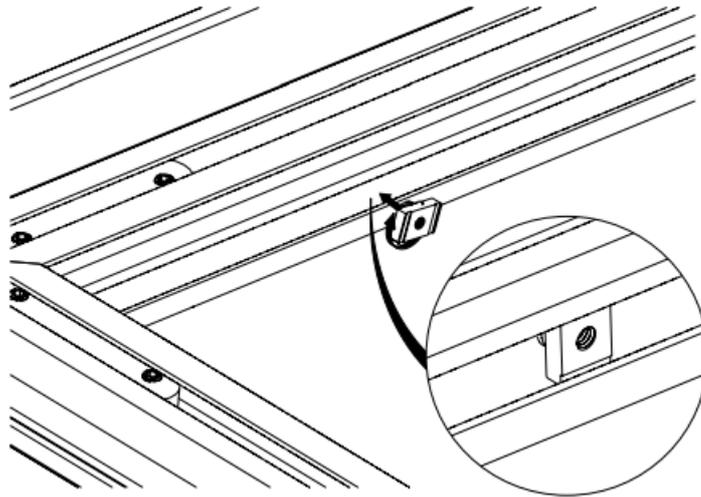
4. Attach the black backer to the inside of the frame through the grommets. Secure with thumb screws.
