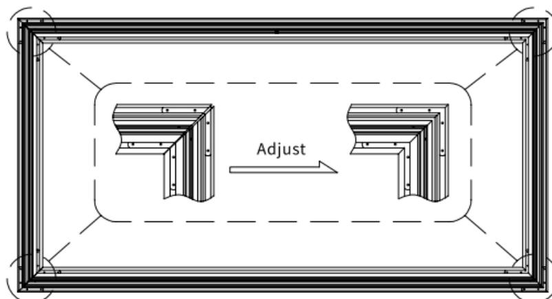
4. Critical Step: Frame squareness is critically importance, refer to the diagram and measure the frame diagonals and compare. If the distance is not within 1/8", push from either side of the longer diagonal until each diagonal is measured within 1/8".
