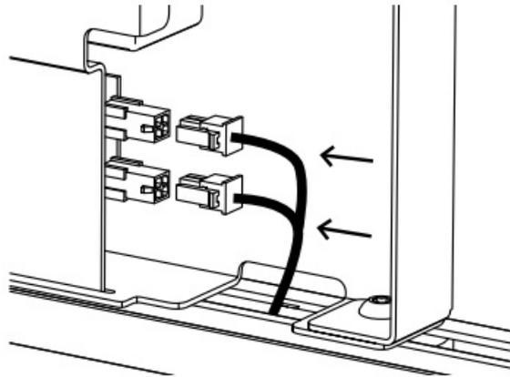
4. Note: Use caution in the next steps; do not kink or fold the light strip, which will cause damage in the circuit. Use the foam strips provided to loosely wrap LEDs around the corners
