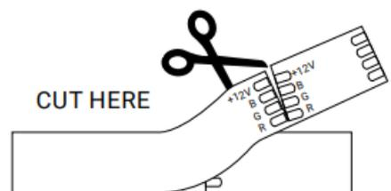
Cut the light strips at the copper pad where indicated to the correct length so they just overlap at the middle of the top frame piece. DO NOT cut the light strips at any other location.
