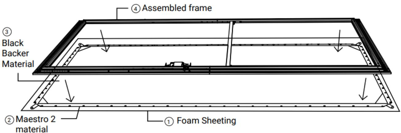
4. Remove and discard the post retention bumpers and distribute the posts along the frame so they align with the holes in the screen's black tensioning media. Refer to the Material Attachment Sequence diagram on page 12 and begin attaching the material to the posts by slipping the holes in the black tensioning media over the post
