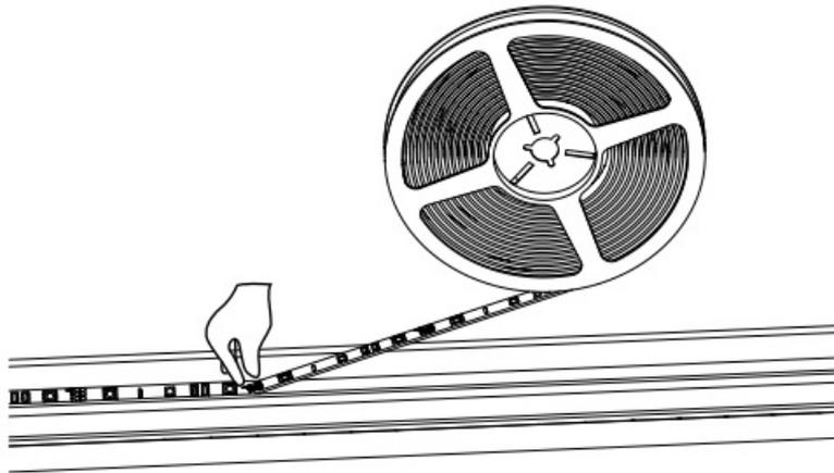
5. Press the lights into the channel on the frame. It is necessary to remove the adhesive backer, the LED strips are securely captured in the LED channel. LED foam must be used when rounding the corners to protect the circuit. Failure to do so will damage the LED strips. The strip should gently round the corner
