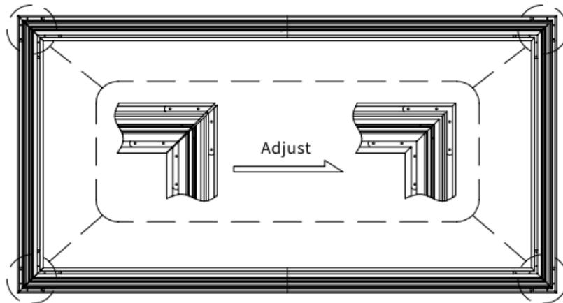
4. Critical Step: Frame squareness is critically important, refer to the diagram and measure the frame diagonals and compare. If the distance is not within 1/8", push from either side of the longer diagonal until each diagonal is measured within 1/8".
