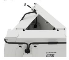
• Route the cable through the cable guidance holes to keep it properly aligned. This prevents accidental disconnection or damage.
