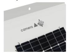
• Attach the scoutlabs Mini to the delta trap using the USB Type-C cable coming from the battery box. Secure the device by clipping the two mounting tabs on the top into place.
