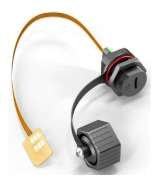
The PI-5 is the suggested optional for installing the SIM injector in a hidden position (e.g. behind a wall/panel). The PI-5 provides a 20cm length flexible tape with SIM card connector and a secure IP67 cap to protect the SIM card slot. Requested mounting hole of M21 with cutoff 19.2mm.
