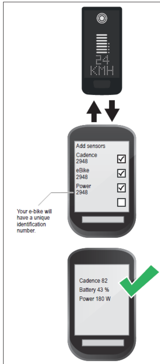
Fig. 8: Connection e-bike to bicycle computer
