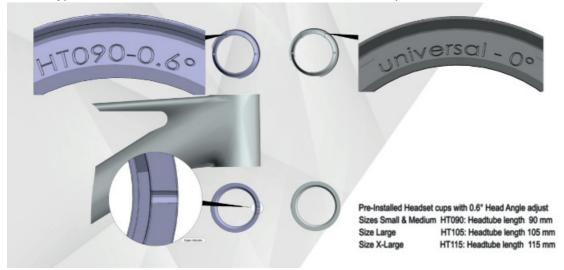
For  $0.6^{\circ}$  this can be installed at + or – but it is essential that the angle indication markers on the headset are set opposite to each other, top facing forward and bottom facing backwards (or vice versa).
