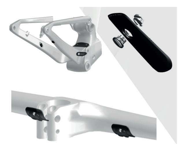
Please be aware that the maximum bolt length for the bottle cage on the seat tube is 10mm. The rivet nuts have closed ends, and using a longer bolt may result in damage to the frame.
