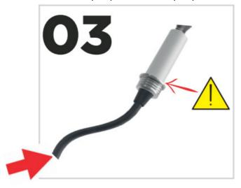
Once the required pressure has been reached, unscrew the lower shock pump head first. Making sure the upper part stays in position.
