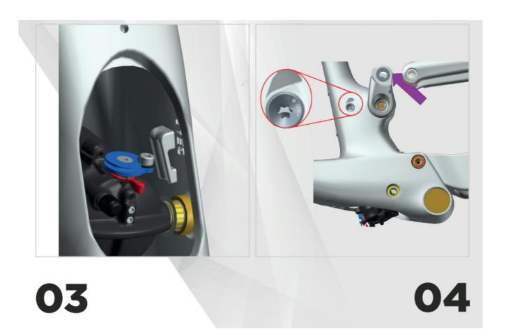
Remove the lower shock bolts and disconnect the TC Cable. Remove the rubber shock bolt cover.
