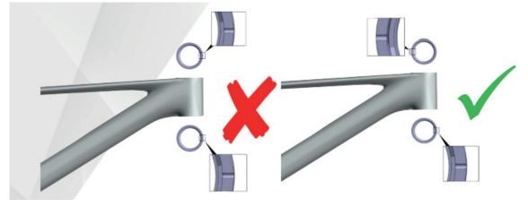
The headset assembly must follow the below no matter which bar/stem system is being used.
