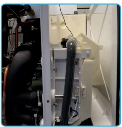
27. Install the white plastic wall. Sanitize this as well before turning the ice machine on and closing the cover.
