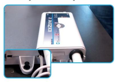
17. Re-attach the Input/Output cover and secure with the original screw.
