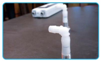
20. Cut and assemble the remaining supply and return tubing and fittings. There should be 12" of unused tubing. Place the handy clamps (black) on the tubing which is placed over the ports on the ICEZONE Unit. Installer's Tip: Heating the tubing in hot water eases the installation of the tubing onto the fittings.
