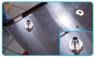
10. The fittings on the top side of the lid should be completed as shown. Ensure the fitting nuts are tight and prepare to mount the ICEZONE unit.
