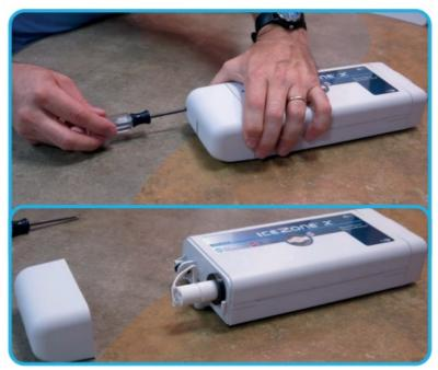
12. Remove the Input/Output cover from the ICEZONE unit. This provides access to additional mounting bosses.
