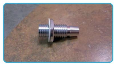
5. Assemble the supply fitting as shown. This includes a single barbed fitting, low profile nut and a white rubber washer.
