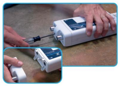
13. Place the ICEZONE Unit on the lid and lay out the routing of the supply and return tubing. The ICEZONE Unit should be placed in the back right corner of the cover (looking at the front of the ice machine). Place the 90-degree hose Barbs in place to visualize the routing. Observe the flow direction arrows on the ICEZONE Unit.
