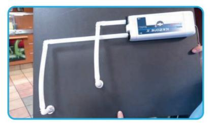
25. Install the top cover. The completed installation on the ice machine should look like the picture shown.
