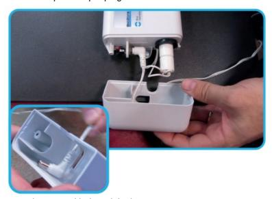
23. Reinstall the service cover and secure with the original screw.
