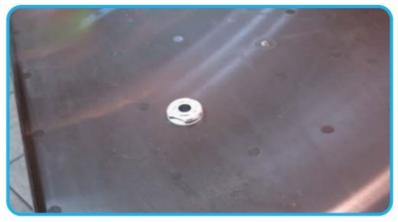
6. Install the supply fitting as shown. This includes a second low-profile nut and a white rubber washer. There should be no exposed threads on the interior surface of the lid per NSF guidelines.
