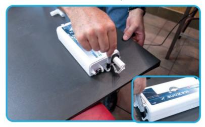
15. Drill the holes to mount the ICEZONE Unit on the lid. Drill three 1/8" holes.
