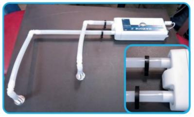
21. Tighten the handy clamps with a pliers to secure the tubing on the ICEZONE unit.
