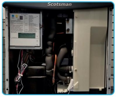
28. Close the ice machine after turning it on. Plug the ICEZONE into a nearby 100VAC outlet that is not switched off. The ICEZONE runs 24 hours/day, 7 days per week. Check to make sure the blue light is lit on the top of the ICEZONE.
