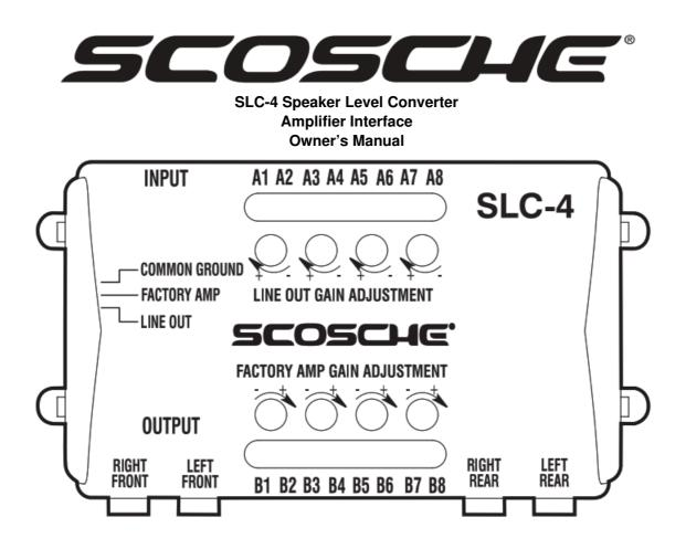
**WARNING:** PRIOR TO INSTALLATION CHECK THAT ALL GAIN LEVEL ADJUSTMENTS ARE SET TO ZERO POSITION. TURN THE ADJUSTMENT COUNTERCLOCKWISE UNTIL IT STOPS.
