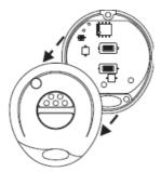
• Remove the discharged batteries and insert the new ones taking care not to invert the polarity.
