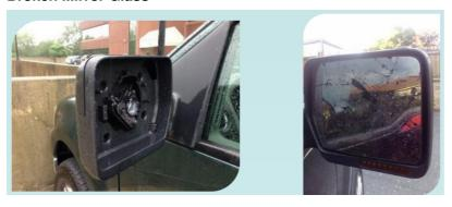
3. If your towing mirror is slightly scratched on your mirror glasses or just the mirror glasses are broken, you need replace the mirror glasses only.
