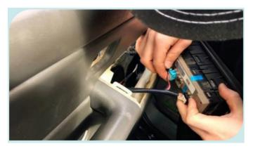
4. Lock the door and fix the screws, then move the plastic plate to the original position and lock the screws.
