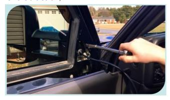
3. Install the new towing mirror out of the window and connect the power cord;
