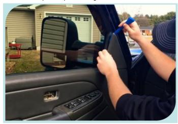
2. Remove the plastic plate to see the rear view mirror and the fixing screw of the door, and use a screwdriver to remove the screw;
