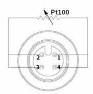
The SciTemp140-M12 is compatible with probes that have the wiring configuration as shown above.
