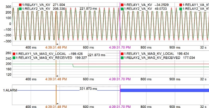
Fig. 11 GOOSE-based magnitude discrepancy detection
