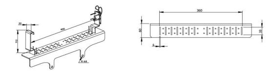
Adjust hooks following cable tray size W100 – 400mm for standart version and 100-400 mm for custom or studio request.
