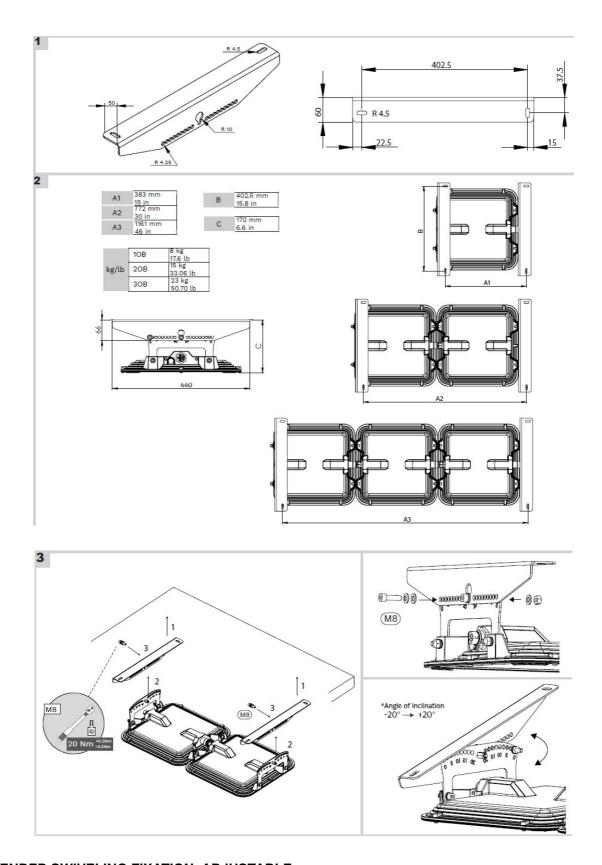
SUSPENDED SWIVELING FIXATION, ADJUSTABLE
