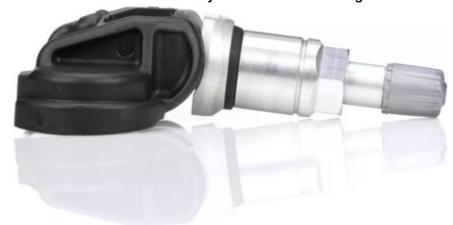
The TPMS Transmitter is installed to the valve stem in each tyre of a vehicle. The unit measures tyre pressure periodically and transmits this information by RF communication to a receiver inside the vehicle. In addition, the TPMS Transmitter performs the following functions:
