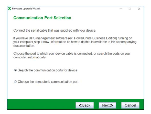
The Firmware Upgrade Wizard will now search the communication ports for the UPS. The UPS is referred to onscreen as the "device". If you have set up virtual ports, it is important to manually select the correct port, the UPS is connected to, here.
