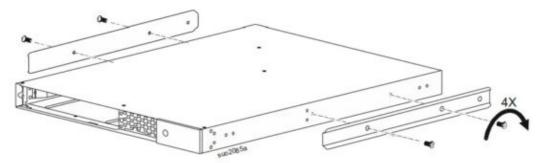
2. Install the rack-mount brackets to the UPS.
