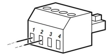
2. Secure the wires by tightening the screws.
