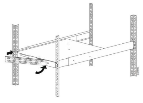
1. Install the rack-mount brackets to the UPS
