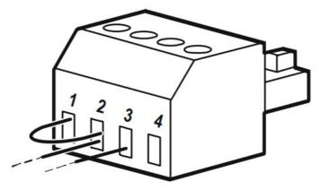
2. Insert a wire jumper between pins 1 and 2. Secure the wires by tightening the three screws at positions 1, 2, and 3.
