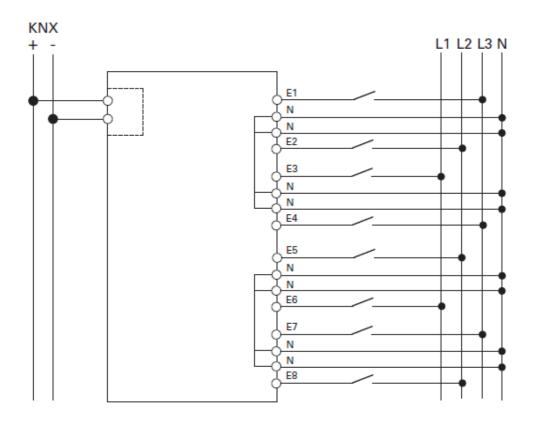
The N conductors must be connected to the device. Inputs E1 to E4 have a common potential  $(4 \times N, \text{ top row})$  and inputs E5 to E8 have a common potential  $(4 \times N, \text{ bottom row})$ . Inputs E1 to E4 and E5 to E8 can be assigned to each other with different phases.
