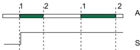
Figure 7 - Operation in Time-Delayed Non-Latching Mode
