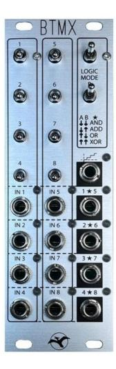
BTMX (BitMix) is a 4-channel selectable logic function module, with each channel having two inputs. All channels share the same logic function and the gateouts are summed with binary weights to create a stepped voltage. Each channel has a switch on the input allowing for hands on control over rhythms or other 4-bit logic signals.
