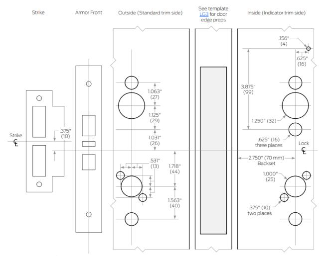
3. Refer to Template LG1 for accurate case and strike dimensions.
