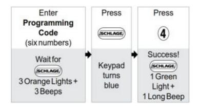
When enabled, no User Codes will unlock the door, preventing any unauthorized attempts of entry when no one is home for a prolonged period of time.
