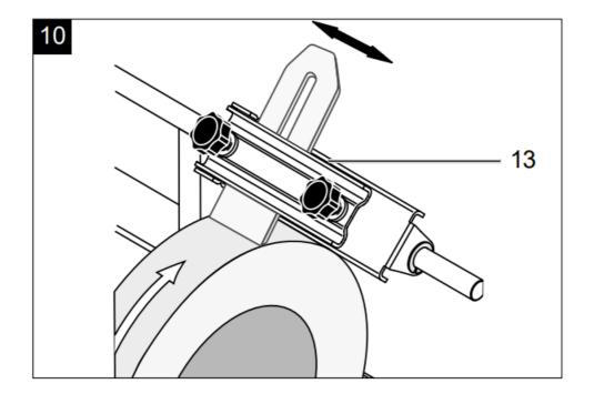
Since the grindstone rotates only slowly, it is possible to detect movement in a lateral direction. This is normal and has no negative influence on the grinding result. Expert tip: New tools still show traces of the production process. You can significantly extend the service life of your tools if you grind them on both sides of the cutting edge before the first use. Simply grind the back in freehand mode on the vertical of the grindstone and the front as follows:
