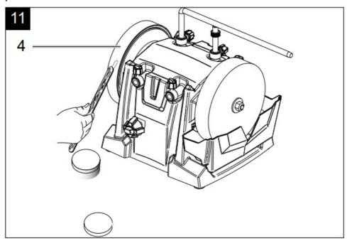
Never sharpen against the direction of the leather honing wheel! Otherwise, the tool will cut into the leather!
