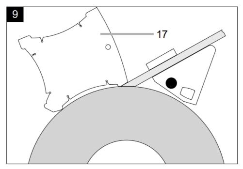
Measure the angle of the workpiece by comparing the cutting edge with the notches. Then set the determined angle on the device by changing the height of the work-piece support. To do so, perform the following steps:
