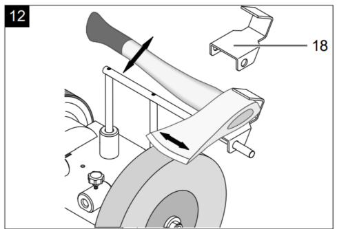
For axes with a length of up to 170 mm. Larger axes are ground without using a grinding support on the tool support.
