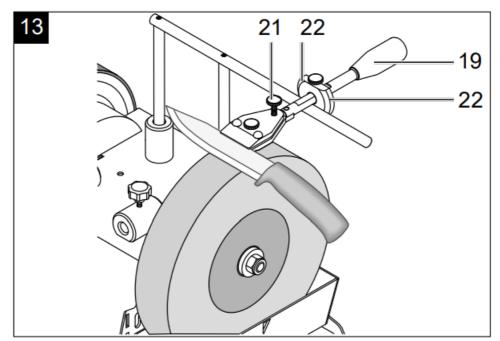
The blade fixtures are designed for blades with a cutting edge of approx. 40 - 100 mm and 100 - 200 mm and for drawing blades.
