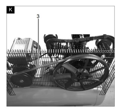
To change the V-belt on the compressor, please be sure to disconnect the device from the mains.
