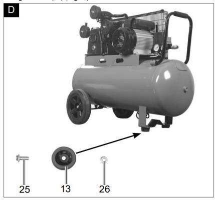
Insert the screw (25) through the foot (13). The foot (13) is subsequently fitted on the mount on the pressure vessel (12). Fasten the foot (13) with the nut (26). Repeat the process for the second foot.
