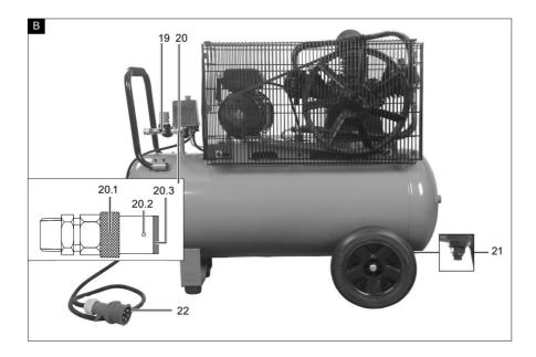
The safety valve (20) is set to the maximum permissible pressure of the pressure vessel. It is not permitted to adjust the safety valve or to remove the connection lock (20.2) between the drain nut (20.1) and its cap (20.3).
