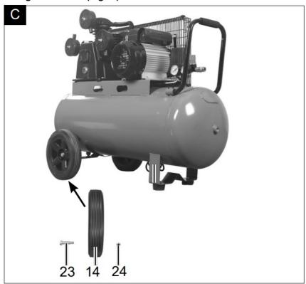
Insert the screw (23) through the wheel (14). Now insert the screw (23) through the mount on the pressure vessel (12). Now insert the screw (23) with the nut (24). Repeat the process on the other side of the pressure vessel (12).
