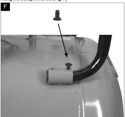
Fasten the transport handle (6) to the pressure vessel (12) with the screw (29) as shown. Repeat this process three times.
