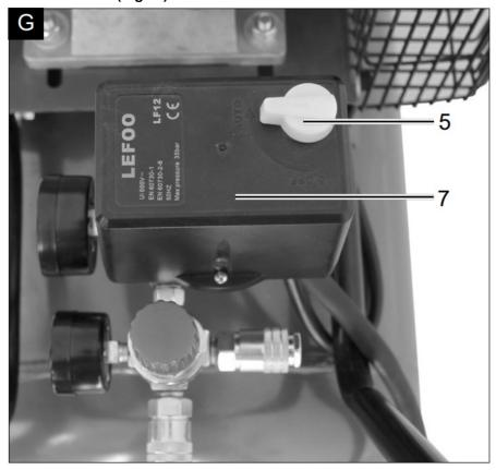
Turn the on/off switch (5) on the pressure switch (7) to the "Auto" position. If the pressure in the pressure vessel (12) is too low, the compressor will start up automatically.
