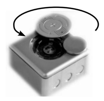
5. Replace the battery by turning the lid on the back of the goniometer counter clockwise.
