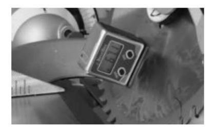
3. Arrest the device on the blade or on the planning arrester by using the integrated magnets (see fig. 2). The goniometer should be held vertically to the table for all measuring activities.
