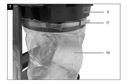
• Attach the dust bag (10) to the lower air outlet using the clamp fitting (11) (fig. 7).
