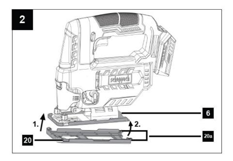
When working on workpiece surfaces that are susceptible to scratches, it is recommended to work with a sliding shoe (20).
