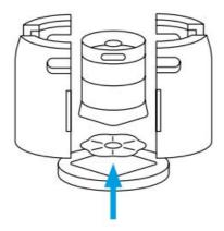
Enclose the chilled KEG in the draft2go insulator jacket to keep the beverage cold for longperiods. Recommendation: place the KEG in the insulator jacket on top of the second pre-cooled ice pack
