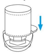
In a few hours, the beverage will now be cooled down to drinking temperature. (See temperature table). At a room temperature of 22° C, the ice sleeve plus ice packs will cool the beverage down to 2-4° C in 2-3 hours.
