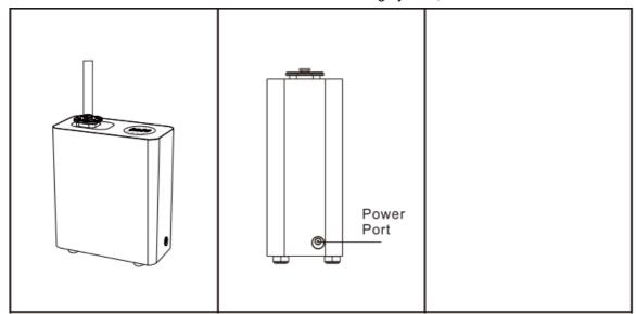
5. Insert the power cord into the power port to power it on and use it.
