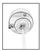
3. It is important to place the pipeline into the correct opening of the nozzle, otherwise the device will not be able to emit odor. There is a small circular pipe bracket inside the nozzle, which needs to be firmly fixed in it.
