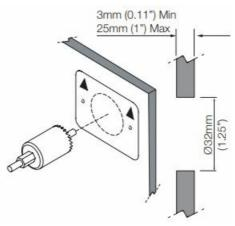
3. FRONT INSTALL ONLY Drill 2 pilot holes for the front fit bezel.
