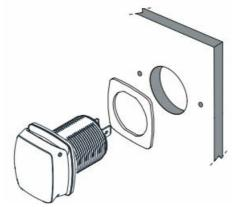
• REAR INSTALL ONLY Tighten the lock ring onto the product until
