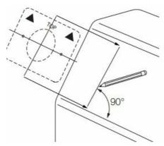
2. Use a drilling template to drill a ø32mm (1 1/4") hole (see tools required).
