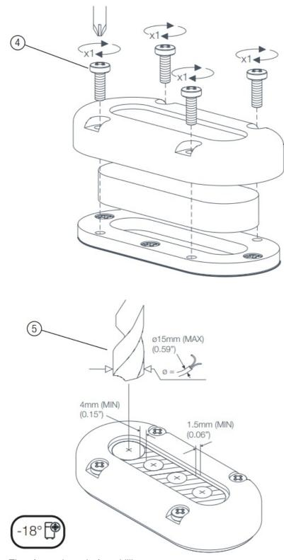
Tip – freeze bung before drilling
