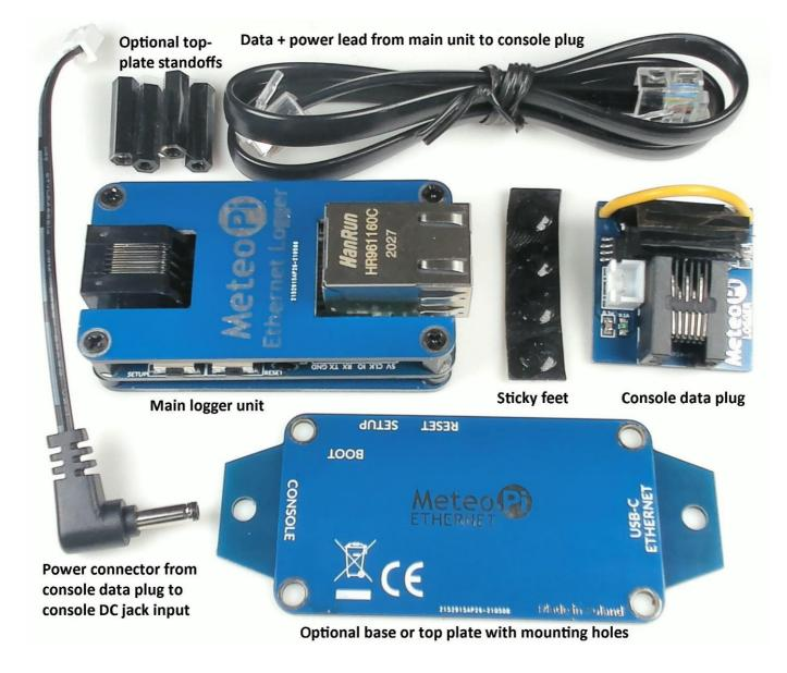
The main logger unit comprises three main parts: There is the main PCB circuit board on which all electronic components are mounted. There is then a base plate and top cover plate attached to the main circuit board by means of screws and standoffs of different sizes – see image below, which shows the default configuration as supplied.
