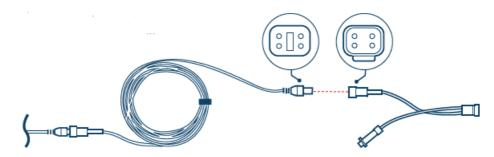
2. Connect your power cable into the other open receptacle of the Y-Power Cable adapter.
