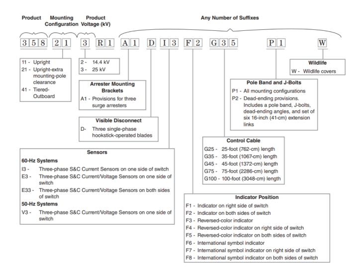
The catalog number created above represents a 25-kV upright-extra mounting-pole clearance Scada-Mate SD switch. It comes with three arrester brackets for one side of the switch, a manual disconnect, and wildlife protection. It also comes with a 60-Hz current sensor and voltage sensors on each side of the switch. To connect to the control unit, a 35-foot (10.7-m) cable option is chosen. A pole band and J-bolts are included.
