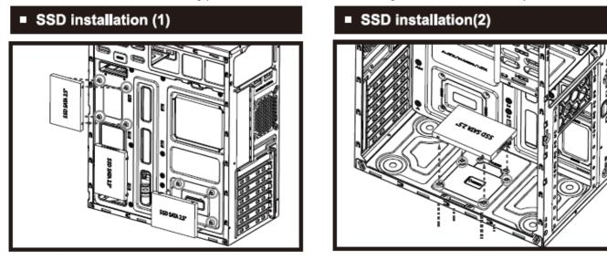
3xSSD can be installed on the M/B bracket as shown in the above illustration 1 x3.5"HDD or 1 x2.5"SSD can be mounted on the bottom cover.
