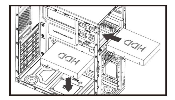
1 x3.S"HDD or 1 x2.S"SSD can be mounted on the bottom cover
