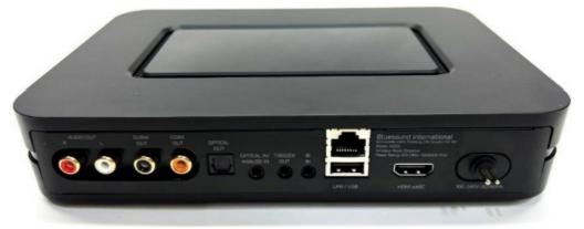
Now the Bluesound Node is ready to be connected to the Sbooster BOTW P&P ECO 5-6V. Before using, please read the manual of the Sbooster BOTW P&P ECO power supply. Please note: the BOTW P&P ECO 5-6V power supply needs to be set on 6V DC output setting The Sbooster AIB includes an active filter. This means that the filter needs power to operate. The output to the Node is a cleaned 5V.
