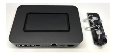
Step 1: Remove the rear cover, which is attached with a magnet.
