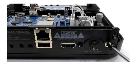
Step 13: Place the top of the enclosure carefully on the bottom then hook the plastic parts in the bottom. Do not damage the tape and wires. When closing you will probably need to push it firmly.
