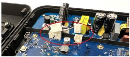
Step 5: Remove 4 screws of the Node's power supply board and take out the metal bracket that covered the connector.
