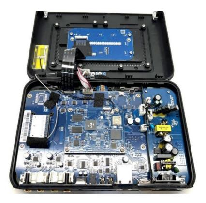
Step 4: Disconnect the white connectors from the sockets.
