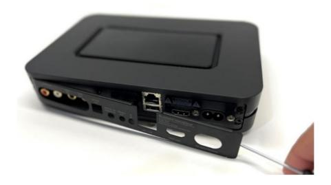
Step 2: Remove 3 screws to unlock the top of the Node.
