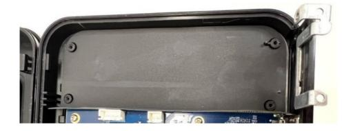
Step 8: Result after removing the internal SMPS and plastic cover sheet.
