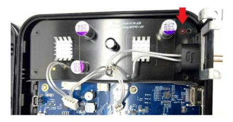
Step 10: Place the mains connector plate over the connector and screw the AIB with 4 screws to the enclosure.
