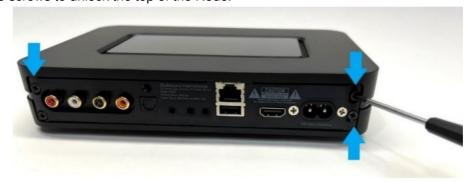
Step 3: Carefully open the top part of the housing by lifting it from the back of the device, until you hear a loud "click". Be careful not to damage the tapes and wires.
