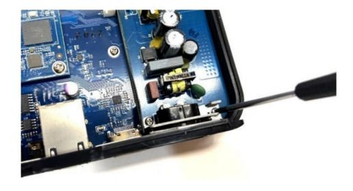
Step 6: Remove 2 screws from the back panel. Then remove the Node's switching power supply board.
