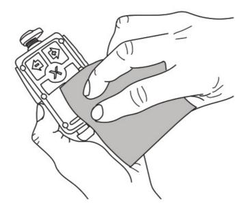
Clean the connectors and use Vaseline spray on the audio connector (female headset plug) twice a year (SAVOX recommends TURBO OIL PRF 290m manufactured by
