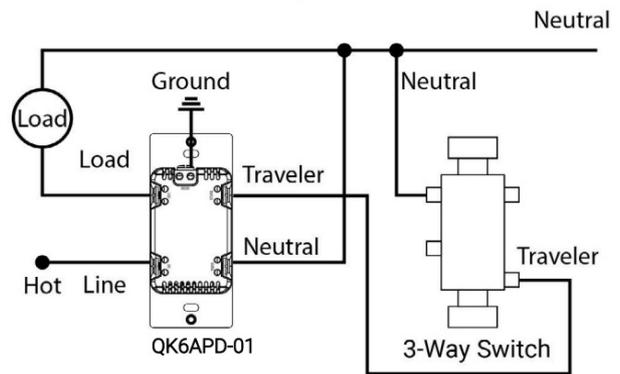
**Note:** For 3-way configurations, ensure the smart dimmer is installed in the junction box where Line (Hot) enters the electrical circuit. Insert wires into holes, do not wrap wires around screws. Do not remove screws. The Qualex 6 Button keypad Dimmer is designed to operate in either 120VAC or 277VAC circuits. For 277VAC 3-way circuits, use standard “off-the-shelf” 277VAC compatible 3-way switch.
